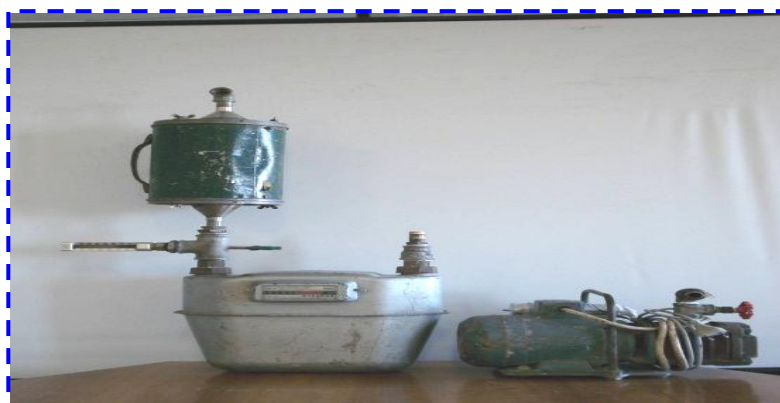
Figure 2: The device used to measure the amount of dust through the chimneys.
